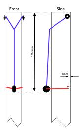
After drilling the holes, use a fid to help guide the rail line in the lower hole and then back out of the upper on both sides (be sure to pass it through the halyard block as well). Tie a stopper knot where the line exits the upper hole to secure the rail line, ensure there is enough slack for the block to sit clear of the mast as show in the picture below.
