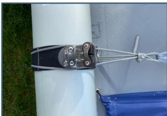
Insert the knot of the provided retrieval bungee (metal ring at other end) into the rear beam track, between the two toe straps. On older boats you may need to remove a hull, but on later boats there is a cut out in the beam slot to make this a simple operation.
