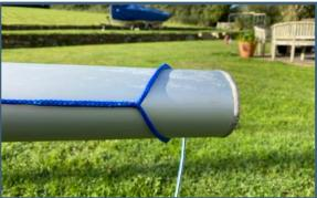
Measure 1750mm down from the mast head, this should be where the halyard block lays. At this level you will need to drill 2 x 5mm holes into the mast track on either side of the section. These need to be 15mm from the trailing edge of the luff groove. This is where the halyard block rail line will attach.
