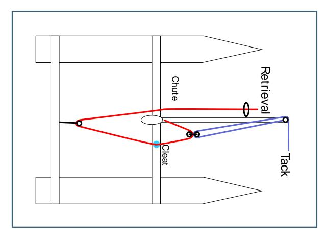
Finally the continuous sheeting system. Starting from the clew of the sail tie one end of the sheet off, then with the other end lead it back to the aft ratchet block on the jib track (be sure to feed it through the correct way). The sheet then goes forward to an additional block (supplied) attached to the jib cleat slider. Continue the lead to the other side of the boat and mirror the arrangement before also attaching the end of the sheet to the gennaker clew.
