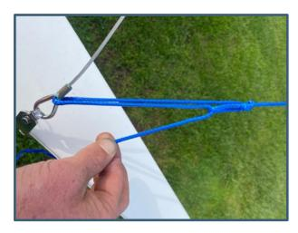
Use the pre-made pole bridal wires to then equally tension the pole to create a small amount of prebend. Use the main bridal eye and the purchase loop to adjust so that the pole remains on the centre line of the boat.
