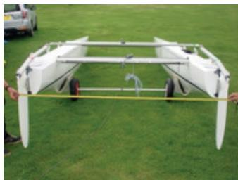
With the stern of the boat supported and the rudders in the down position adjust the screw until the rudder blades are in line with the keel. (Fig 10)
